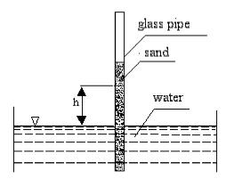
Diagram presenting the capillary rise of water through sand Lithomex has a very low degree of Capillarity. Porosity - defines the amount of holes (pores) in the unit of the material volume and can have a bearing on the durability and breathe-ability of the masonry and the repair material. The porosity of the masonry and the repair material is a function of the Pore size
